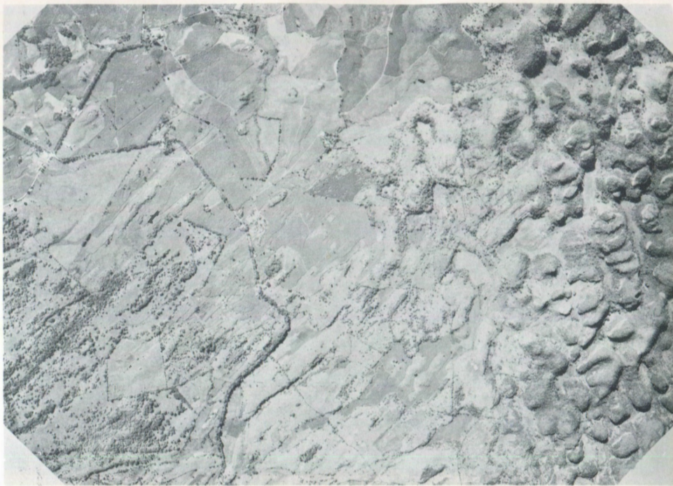
Figure 14. Vertical aerial photograph of area underlain by Lares Limestone from 2.1 to 4.5 kilometers west-northwest of Morovis. Thin-bedded limestone in eastern two-thirds of area weathered to zanjon karst; massive limestone along strike in western third weathered to cockpit or cone karst.
